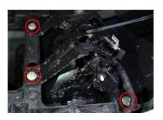
2. Access your factory fog lights and unplug the fog lamp connector. Use a 10mm socket and ratchet to remove the three bolts, as shown in the picture to the left. Remove the factory fog light housing. The factory bolts will be reused.
