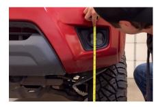
8. On your vehicle, measure the distance between the ground and the center of your SS3 pod. This is your mounting height.
