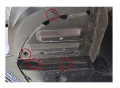
3. Use a plastic trim removal tool to remove the four push rivets on the outer splash guard. Gently pry the splash guard down to gain access to the fog lights. The splash guard will still be connected to the inner fender liner. It should not be necessary to completely remove it unless desired.
