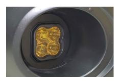
5. Using the OEM hardware, loosely install the bracket and pod in the fog pocket. Install the nuts hand-tight and do not snap the push rivets down as the pod will need to be removed to lock-in final aiming.
