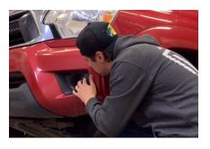
9. Loosen the 5/32" allen bolts on each side of your SS3 pod, just enough to allow you to adjust the pod.
