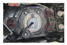
4. Remove the factory fog light assembly. Use a T20 Torx driver to remove the three screws. We recommend using hand tools to reduce the chance of thread stripping or heating of the plastic that may occur with power tools.
