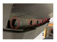
2. Using a trim removal tool, remove the eight push rivets along the front of the splash guard. We recommend prying on both accessible sides of the push rivets at the same time due to their large size.
