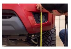
10. On your vehicle, measure the distance between the ground and the center of your SS3 pod. This is your mounting height.
