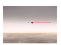
14. Aim your SS3 pods on each side, so that the top of the beam pattern is on the cutoff line mark.
