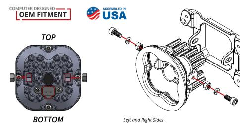
1. Install the supplied nuts into the pod housing with the nylon facing inward. Attach the bracket to the pod using the supplied screws and washers. Make sure the bracket is in the correct orientation. See diagrams above. Ensure that the screws are tightened such that the pod retains its position, but can pivot with force for aiming.
