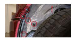
2. Peel back the wheel well fender liner. To do so, remove the two push clips, two 5.5mm bolts, and two 7mm bolts shown in the picture to the left and peel the fender liner back.
