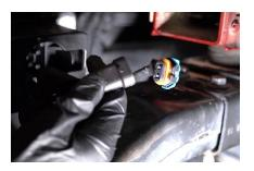
10. Reinstall the factory fog light bezel, by reinstalling the factory hardware. Plug the SS3 into the factory fog light harness using the included DT wire adapter. Test function. If the light does not turn on, try flipping the connector 180°.
