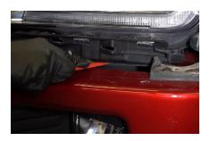
5. Remove the shroud blocking access to the fog light bezel. To do so, remove the 10mm bolt and loosen the three plastic pins holding the shroud to the bottom of the headlight. Then remove the two 10mm bolts near the fender flare. Remove the shroud from the vehicle.
