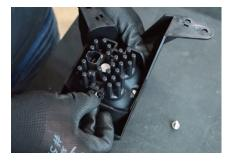
1. Install the supplied nuts into the pod housing with the nylon facing inward. Attach the bracket to the pod using the supplied screws and washers. Make sure the bracket is in the correct orientation. See diagrams above. Ensure that the screws are tightened such that the pod retains its position, but can pivot with force for aiming.
