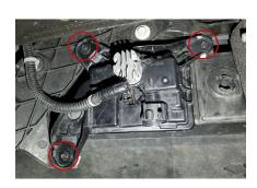
3. Use a 7mm socket and ratchet to remove the three bolts holding the factory fog light housing in place, as shown in the picture to the left. Remove the factory fog light housing. The factory bolts will be reused.
