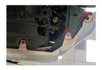
3. Using a 10mm socket, remove the six screws along the bottom of the bumper (passenger's side shown in picture to the left).
