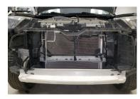
6. With help from a second person, pull the bumper straight forward to release snaps around the headlights and remove the bumper.
