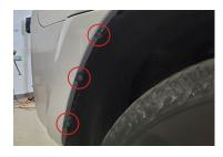
4. Using a 10mm socket, remove the three screws from the edge of the front bumper in the wheel well.
