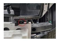
8. Using a 14mm wrench, loosen the second from the outboard bolt on the bumper bar (driver's side shown in picture to the left).
