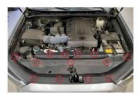
1. Remove the thirteen push-rivets holding the core support trim panel in place. Push down in the center of each push-rivet and then use a plastic trim removal tool or flathead screwdriver to extract the push-rivet.
