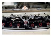
2. Using a trim removal tool or flathead screwdriver, remove the six plastic push-rivets shown in the image to the left.
