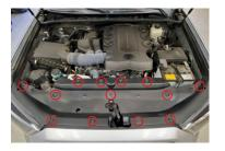
7. Reinstall the core support trim panel using the original thirteen push-rivets. Push the center of the push-rivets down so that they are flush with the top of the surface to lock them in place.
