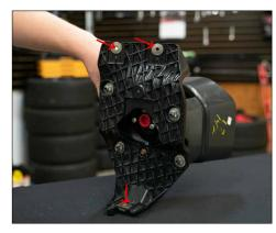
**2.** With the metal brace removed you can remove the entire foglight bracket assembly by removing the three 8mm bolts shown above.
