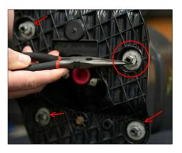
**3.** Set the foglight bracket assembly on a table. Remove the four metal retaining washers using a pick or flathead screw driver. Then remove the four 13mm nuts that secure the front bezel to the foglight bracket.
