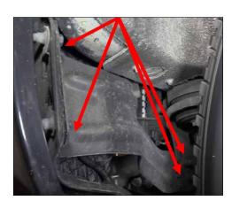
**12.** Finish the installation by reinstalling the metal brace using the four 13mm bolts removed in Step 1.
