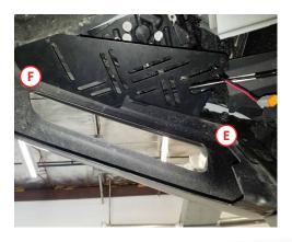
3. Slide the bracket in-between the bumper and the support (). Using the stock mounting points, replace the original 13mm screw, only hand-tightening it.
