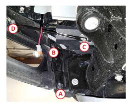
1. Using a 13mm socket, loosen screw (a). Do not fully remove the screw. Next, remove screw (b).
