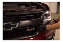
6. Remove the bumper and grille by pulling straight out from the vehicle and releasing the two push tabs securing the bumper to the front of the vehicle. Set the bumper and grille aside on a soft surface.
