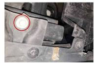
4. From underneath the truck, remove the two 10mm hex bolts securing the bumper to the frame of the truck.
