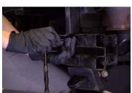
9. Reinstall the crash bar using the original 15mm bolts. Secure the bolts to 43 foot pounds.
