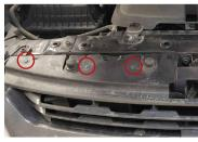
3. Remove the six T15 torx screws holding the top of the grille to the radiator core support.
