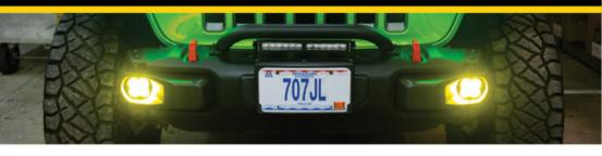
Thank you for your purchase of our new SS3 Type MR Foglight Brackets. CAD-designed to use existing mounting points, this kit allows you to mount Diode Dynamics SS3 LED Pods in the factory foglamp location on JK and JL Jeep Wrangers with factory-installed steel bumpers.
