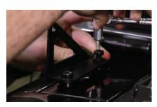
3. Align the bracket in place, and use the included OEM-style extended hardware to secure. Repeat for the other side of the vehicle.
