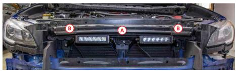
4. With the bumper removed, locate and remove the 12mm bolt (a) in the center and the two 10 mm bolts on the sides (b).
