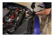
1. Using a 10mm socket and plastic trim removal tool, remove the six bolts and four plastic rivets located on the edge of the bumper inside the engine bay.
