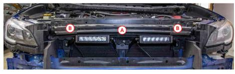
4. With the bumper removed, locate and remove the 12mm bolt (a) in the center and the two 10 mm bolts on the sides (b).
