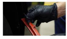
**6.** Disconnect the OEM sidemarker. Then install your new sidemarker. Test for function and secure using the two T25 torx screws.
