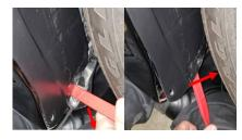
**3.** Push down on the flap secured to the fender liner and pull the fender liner toward the wheel to separate from the flap.
