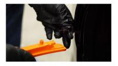
**5.** Disconnect the OEM sidemarker. Then install your new sidemarker. Test for function and secure using the two T25 torx screws.
