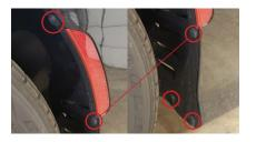
**1.** Remove the four push clips securing the fender liner to the bumper.
