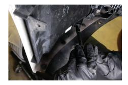
**3.** Looking at the fog light bezel, unplug the factory turn signal, sidemarker, and fog light connectors by depressing and pulling straight back. Then remove the six 7mm screws holding the fog light bezel in place.
