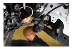
**13.** Then connect the red wire from the turn signal housing to the spade connector on the wiring harness.
