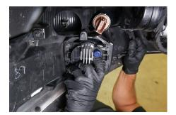
**4.** Press outward on the tabs holding the fog light bezel in place to separate it from the bumper. Once the bezel has been removed, take it to a working area with a soft surface.
