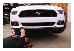
**2.** Remove the belly pan from underneath the vehicle. To do so, remove the 12 7mm screws on the outside edge, four 7mm screws on the belly pan itself, and six plastic rivets on the outside edge to remove the belly pan.
