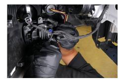
**11.** Plug the connector on the turn signal housing into the factory turn signal connector. Then reconnect the sidemarker and fog light connectors.
