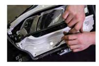
1. Remove the four T20 screws holding the lower optics shroud and light pipe in place.
