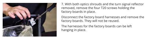
8. Install your new Diode Dynamics LED boards using the original screws.
