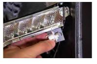
10. Reinstall the lower retaining clips that were removed from step 3 to the LED Boards.
