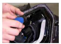
1. Remove the six T20 torx screws holding the black bezel in place, including the screw on the backside of the housing. Set the bezel aside.
