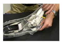
1. Remove the lens and set the headlamp assembly aside. Next, remove the 3 screws holding the bezel to the lens. Then remove the bezel from the headlight lens.
