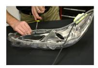
6. Using a microfiber cloth, remove any finger prints that may be on the bezel then reinstall it back into the headlight lens by clipping it into place. Reinstall the original screws.
