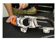
4. Install your new Diode Dynamics C-Light by running the wires through the hole where the factory bulb was and setting the LED board into place.
