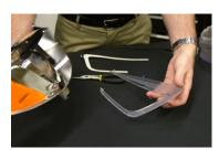
3. Pull the reflector lens straight out to remove it and set it aside.
