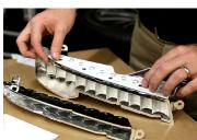
3. Remove any shavings from the reflector housings. Using the original plastic rivet points, place the new Diode Dynamics LED boards into position.
