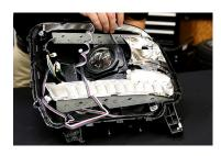
7. Run the switchback ribbon cable out of headlamp, sealing any hole that you may create. Replace the headlamp lens and repeat for the other side.
