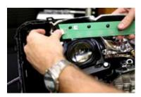
1. Remove the headlamp lens. Using a T20 Torx Screw Driver, remove the screws holding both reflector housings in place to access the factory LED panels. Pull the reflector housings away from the headlamp and unclip each connector.
