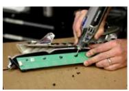
2. Take both reflector housings to a clean area. Using a rotary (Dremel) tool, remove the factory LED boards by shaving down the black plastic rivets holding the LED panels to the housing. Pull the factory board away from the housing. Repeat for all three factory boards.
