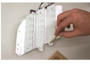
5. Fix the new panels in place by applying epoxy or other permanent adhesive where the plastic rivets were shaved down. The epoxy should create a bond between the plastic rivet point and the board. Use enough epoxy so that there is a bond all the way around the rivet, contacting the board fully.
