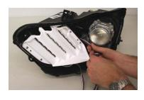
7. Run RGBW ribbon cable out of headlamp, along with the 6-lead sequential connector, sealing any holes that you may create.
