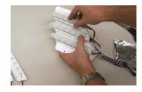
4. Place the new Diode Dynamics LED boards into position. All holes should align perfectly. Due to the larger footprint of the new LEDs, the panels will not push down fully in place. One of the LEDs in each segment may be partially obstructed by the white housing. This is normal fitment, as intended.
