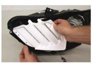
6. Once the epoxy is fully set, reinstall the black panel and white bezel to the main headlight housing using the original screws.
