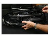
7. Using the alignment tabs, reinstall the black bezel. Once complete, replace the original torx screws and headlamp lens. Repeat for other headlamp.
