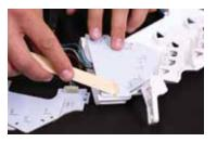
5. Place your new Diode Dynamics LED boards into position. All holes should align perfectly. Secure the new boards in place by applying epoxy or other permanent adhesive where the plastic rivets were removed. The epoxy should create a bond between the plastic rivet mounting point and the board. Use enough epoxy so that there is a bond all the way around the rivet, contacting the board fully. We recommend securing the board labeled 3 first and working your way forward.
