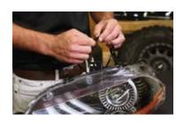
7. Run the wiring out of headlight, sealing any holes that you may create.
