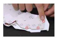
4. Bring the DRL bezel to a clean area. Using cutting pliers, remove the three plastic rivets holding each LED board to the bezel and remove the LED boards.
