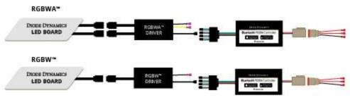
IMPORTANT: DO NOT plug the LED panel directly into controller without the driver. The LEDs must be plugged into driver first to control the power.
