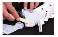
5. Place your new Diode Dynamics LED boards into position. All holes should align perfectly. Secure the new boards in place by applying epoxy or other permanent adhesive where the plastic rivets were removed. The epoxy should create a bond between the plastic rivet mounting point and the board. Use enough epoxy so that there is a bond all the way around the rivet, contacting the board fully. We recommend securing the board labeled 3 first and working your way forward.
