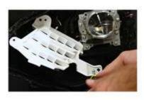
Once the epoxy is fully set, reinstall the white bezel to the main headlight housing using the original screws.
