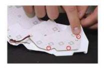
Bring the DRL bezel to a clean area. Using cutting pliers, remove the three plastic rivets holding each LED board to the bezel and remove the LED boards.
