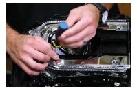
2. After the headlight has been opened, remove the four Phillips screws holding the silver bezel in place. Remove the silver bezel and set it aside on a soft surface.
