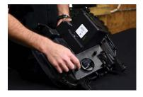
1. Before opening the headlight, remove the three Phillips screws holding the HID ballast in place and four Phillips screws around the edge of the headlight. Then remove the HID ballast.
