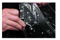
3. Remove the four Phillips screws holding the factory optic assembly in place. Then remove the factory optic assembly and disconnect the two factory board connectors. These connectors will not be reused, so tuck them out of the way.
