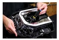
6. Route the wire outside of the headlight, sealing any holes you may create. Reinstall the silver bezel using the original screws. Repeat the process for the other headlight.
