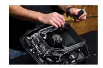
4. Reinstall the factory optic assembly using the original screws.
