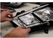
2. Unclip the factory connector and pull the LED panel housing straight out to remove it. Set the rest of the headlamp housing aside.
