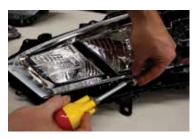
1. Remove the lens. To access the factory LED panels, remove the 3 Phillips screws holding the panels to the black plastic housing.
