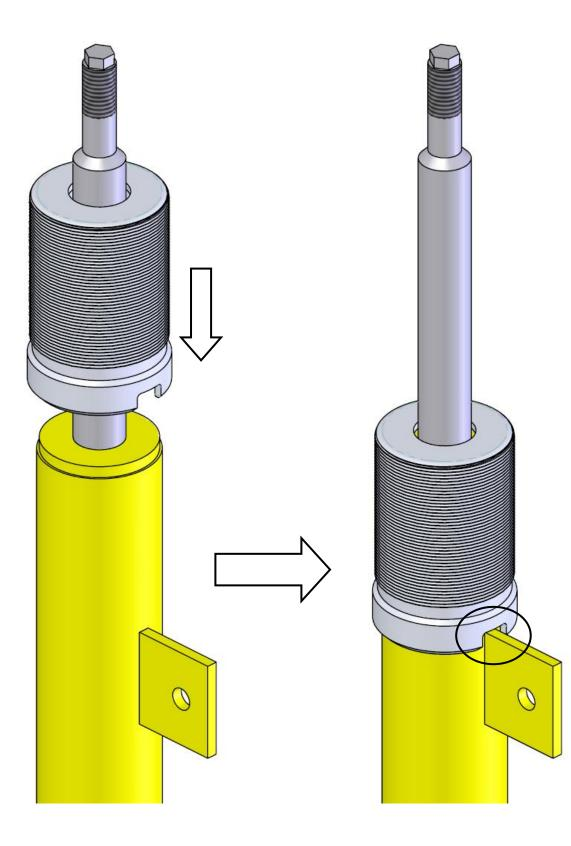
6. Install the spring perch and black plastic isolator disc (in Coil-Over Hardware Kit) as shown. Adjust the perch to its lowest setting. This will be the starting ride height setting, and should get you very close to Dinan's target bumpstop clearance measurement. Snug the 6mm screw to lock the perch into place.
