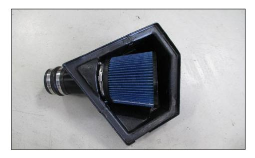
14. Attach the Dinan intake tube and silicone hoses using the included hose clamps as shown below. Leave the hose clamps slightly loose for now, so the intake tube can be adjusted into position later.
