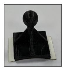
21. Snap the ball joint mount into the mounting hole of the plate that will sit over the airflow meter tube. This is to replace the mount that was removed with the stock airbox.
