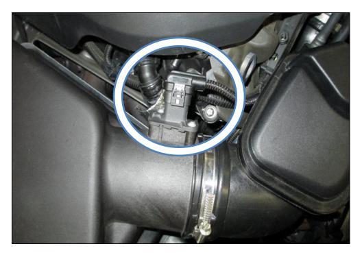
3. Release the four clips holding the airbox lid in place.
