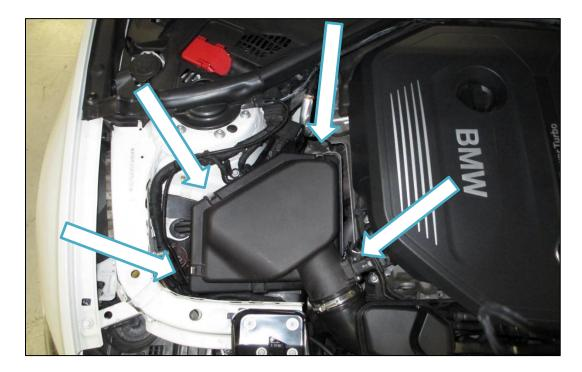
4. Follow the outlet of the airbox, down to the hose clamp near the turbocharger inlet. Loosen this hose clamp.
