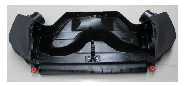
4. Install the Dinan air filters as shown. The open end of the Dinan air filters will slide inside the oval openings in the air box. The rubber "block" on the air filter cap points downward and helps hold the filters away from the air box bottom.
