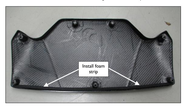
8. Place the Dinan lid onto the airbox. Be sure there is no foam strip visually exposed once the lid is installed, as shown in the next two figures.
