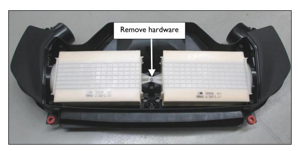
3. Remove the factory air filters.
