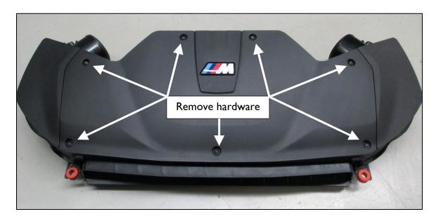
2. Remove the screw in the center of the airbox that fastens the factory air filters. Save this screw for installation of the Dinan Cold Air Intake.
