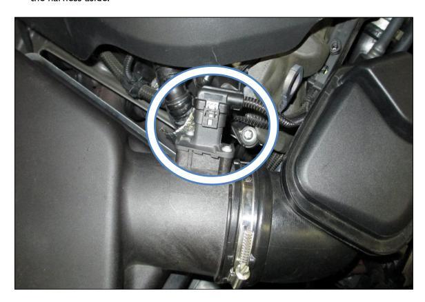
3. Use a Torx tool to remove the two screws holding the sensor in place and remove the sensor. Do not drop or damage the sensor as it is very fragile. Set sensor aside. It will be reinstalled later.
