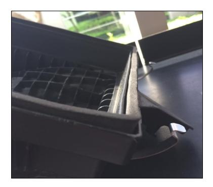
13. Referring to the figure below, attach the Dinan air mass meter to the carbon airbox lid using the 5mm bolts, round & rectangular washers, and nuts as shown. The air mass meter only fits one way.
