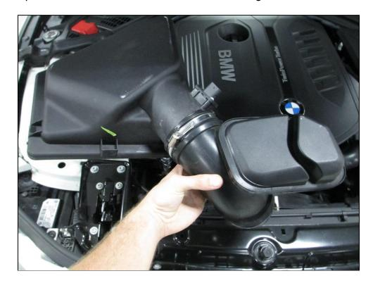
7. WARNING – the turbocharger inlet is now exposed. Items which fall inside can cause severe damage to the turbo! Be sure to place a rag or towel in the inlet to protect the turbo.
