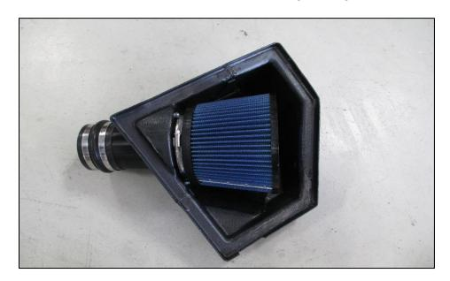
15. Attach the Dinan intake tube and silicone hoses using the included hose clamps as shown below. Leave the hose clamps slightly loose for now, so the intake tube can be adjusted into position later.
