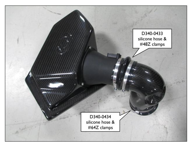
16. Remove the rag from the turbocharger inlet, and install the Dinan intake into the vehicle. Adjust positioning of the intake tube to best clear the radiator bracketry (see below).
