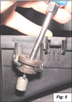
8. Remove the stock Air box top from the assembly by opening the clips. Remove the charcoal evaporative filter that is clipped to it by carefully prying
