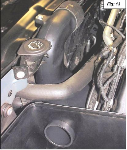
13. Follow BMW TIS instructions to remove the front bumper to gain clearance to install the air duct inlet that picks up high-pressure air in front of the radiator on the passenger side. See figure 14.
