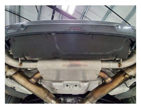
15) Push the muffler up and forward then torque the clamps. If the muffler contacts any part of the car, twist the inlet pipes to adjust. Allow for the pipe clearances as pictured below.
