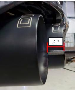
17) After adjusting the tip length and alignment, make sure the second vertical line of the N in the Dinan logo is facing straight up on all 4 tips.
