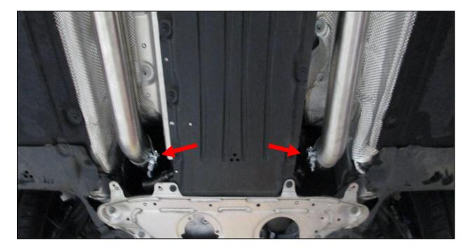
7. Push each pipe forward up against the lip, so that there is NO gap between the Dinan pipe, and the outlet from the engine.
