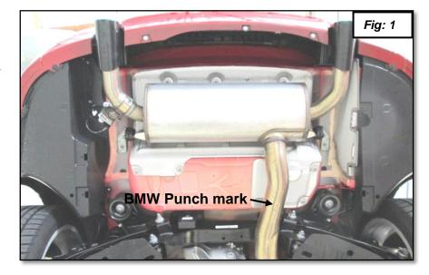
2. This step applies to F22 M240i, F30/F34 335i/340i, F32 440i Coupe, F33 435i & 440i Convertible, F36 435i & 440i Gran Coupe only; skip to step #4 if you are working on a F32 435i Coupe. For a M240i/335i/340i/440i Coupe/435i Convertible & Gran Coupe, cut off the stock muffler at the punch mark as shown in figures 1, 2, and 3. Mark the cut line.
