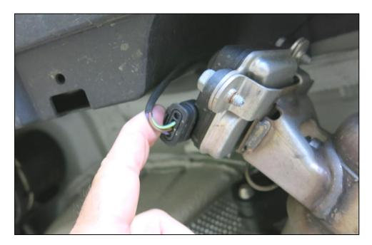
6. Support the stock muffler with a stand and remove the nut on each side of the muffler holding the hanger brackets to the chassis.
