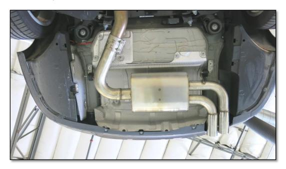
2. Locate the stock BMW Punch mark on the underside of the inlet tube to the stock Muffler.
