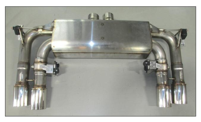
I. Disconnect both valve actuators.
