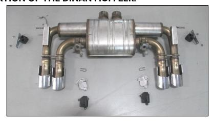
5. There are two types of DINAN exhaust valves. Examine the following diagrams to determine which type is on your DINAN exhaust. Using the hardware provided, install the valve actuator mounting brackets, as shown in the appropriate diagrams.
