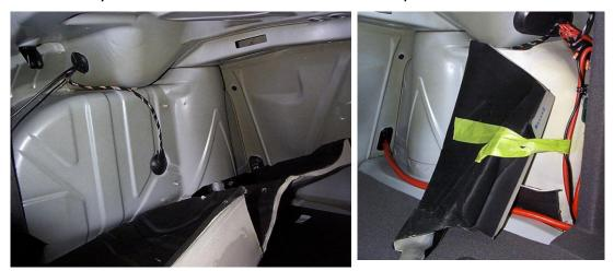
10. Carefully fold the sound insulation backward to expose the shock towers.
