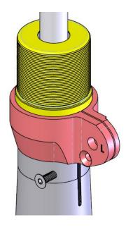
12. Install the spring perch and black plastic isolator disc (in Coil-Over Hardware Kit) as shown. Adjust the perch to its lowest setting. This will be the starting ride height setting, and should get you very close to Dinan's target bumpstop clearance measurement. Snug the 6mm screw to lock the perch into place.
