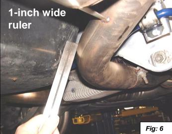
Tighten the clamp to specified torque:
