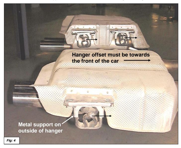
6. Insert the original mounting bolts into the hangers and carefully install both heat shields (with the two inner hangers and one outer hanger on each side). Use the stock nuts you removed in step 2 to fasten to the car. You need to make sure the bolts don't fall out when you install the hanger-shield assembly. Note: the inner bolts can't be installed after the mounts are in place.
