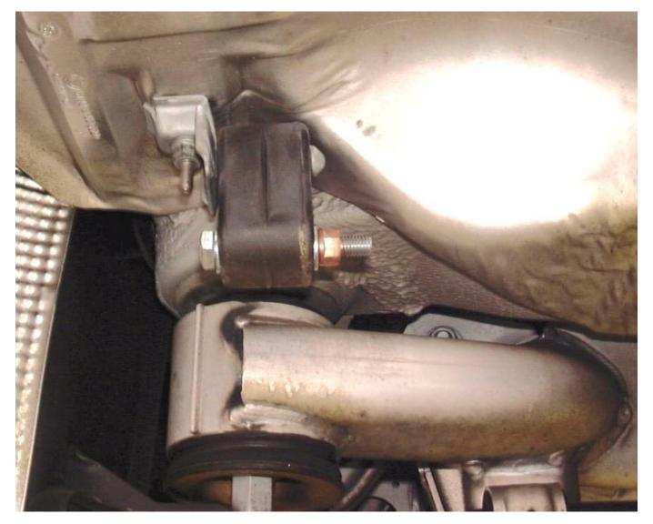
4. Install the hanger onto the car as shown.
