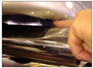
The clamp alone may be removed by cutting the tack weld revealing four slots underneath **or** cut off the entire clamp assembly flush with the back of the clamp.
