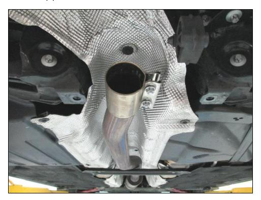
5. With DINAN exhaust secured on a jack or stand, put the muffler in place. When mounting the muffler it should be held with the tips up near the bumper and the muffler pushed forward against the end of the stock pipe.
