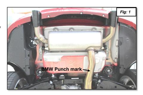
2. This step applies to F22 M240i, F30/F34 335i/340i, F32 440i Coupe, F33 435i Convertible and F36 435i Gran Coupe only; skip to step #4 if you are working on a F32 435i Coupe. For a M240i/335i/340i/440i Coupe/435i Convertible & Gran Coupe, cut off the stock muffler at the punch mark as shown in figures 1, 2, and 3. Mark the cut line.
