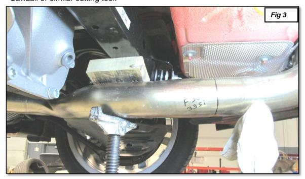
4. This step applies to F32 435i Coupe only; skip to step #6 if you are working on a F22 M240i, F30/F34 335i/340i, F32 440i Coupe, F33 435i Convertible, or F36 435i Gran Coupe. For a 435i coupe, find the BMW factory punch mark on the exhaust. Measure ¾ of an inch from the punch mark toward the back of the car and cut at that point.
