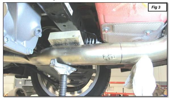
4. This step applies to F32 435i Coupe only; skip to step #6 if you are working on a F30/F34 335i/340i, F33 435i Convertible, or F36 435i Gran Coupe. For a 435i coupe, find the BMW factory punch mark on the exhaust. Measure ¾ of an inch from the punch mark toward the back of the car and cut at that point.
