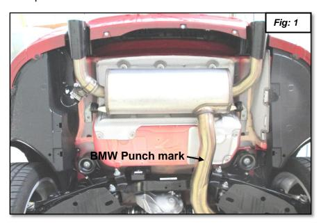
2. This step applies to F30/F34 335i/340i, F33 435i Convertible and F36 435i Gran Coupe only; skip to step #4 if you are working on a F32 435i Coupe. For a 335i/340i/435i Convertible & Gran Coupe, cut off the stock muffler at the punch mark as shown in figures 1, 2, and 3. Mark the cut line.
