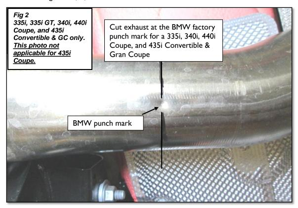
3. Support the stock muffler with a jack or stand. See figure 3. Use a Sawzall or similar cutting tool.
