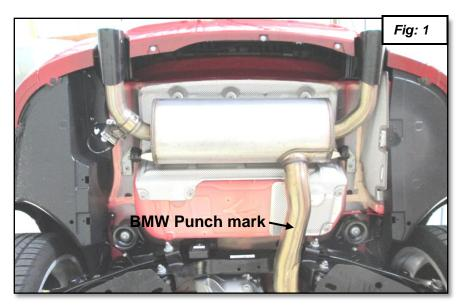
2. This step applies to F30/F34 335i/340i, F32 440i Coupe, F33 435i Convertible and F36 435i Gran Coupe only; skip to step #4 if you are working on a F32 435i Coupe. For a 335i/340i/440i Coupe/435i Convertible & Gran Coupe, cut off the stock muffler at the punch mark as shown in figures 1, 2, and 3. Mark the cut line.
