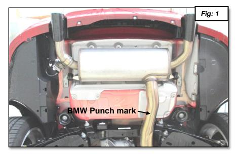
This step applies to F30/F34 335i/340i, F32 440i Coupe, F33 435i Convertible and F36 435i Gran Coupe only; skip to step #4 if you are working on a F32 435i Coupe. For a 335i/340i/440i Coupe/435i Convertible & Gran Coupe, cut off the stock muffler at the punch mark as shown in figures 1, 2, and 3. Mark the cut line.
