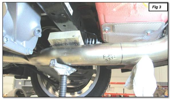
4. <u>This step applies to F32 435i Coupe only</u>; skip to step #6 if you are working on a F30/F34 335i/340i, F32 440i Coupe, F33 435i Convertible, or F36 435i Gran Coupe. For a 435i coupe, find the BMW factory punch mark on the exhaust. Measure <sup>3</sup>/<sub>4</sub> of an inch from the punch mark toward the back of the car and cut at that point.
