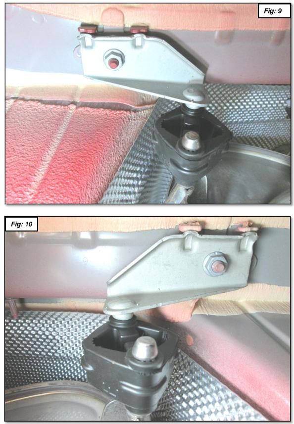
8. Remove nuts holding the hangers to the body as shown in figures 9 and 10 and remove the muffler.
