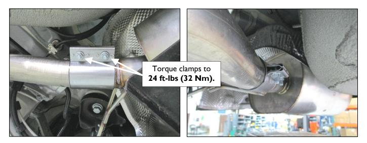
8. Use the stock cross brace located in front of the mufflers for additional adjustment.
