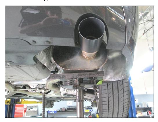
6. With muffler held in place, tighten front and rear hangers, torque to 15 ft-lbs (21 Nm).
