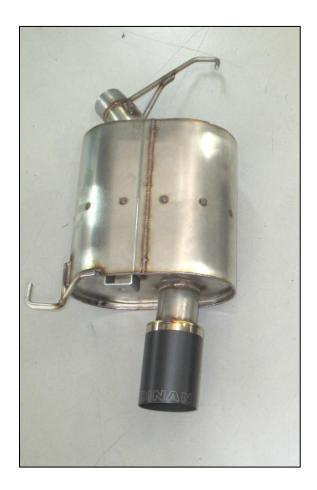
I. Support the muffler securely with a jack or a stand, locate the dimple on the stock pipe then cut the stock muffler as shown in **Figures I & 2**. Before cutting the stock muffler, hold DINAN muffler underneath stock muffler to verify the stock pipe will not be cut too short!
