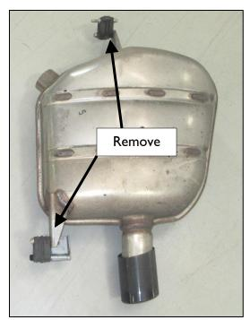
4. Install rubber hangers and stock weight onto DINAN mufflers as shown.
